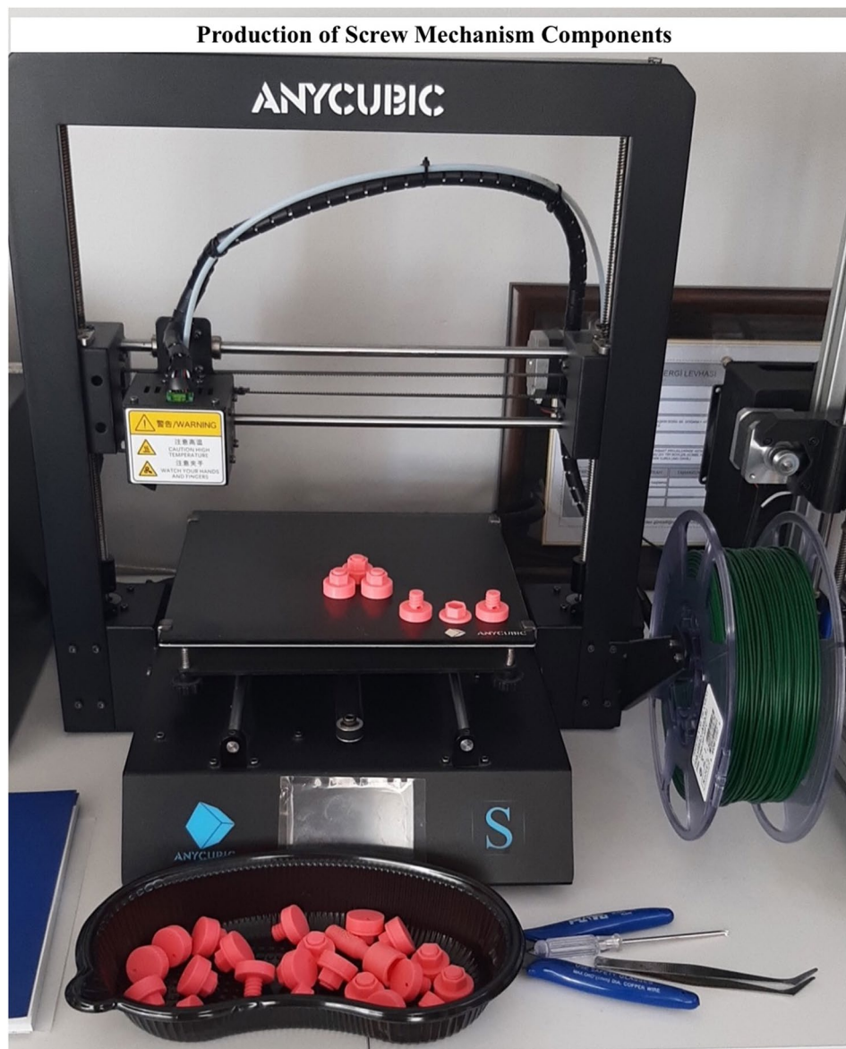
Fig. 3 Production of screw mechanism components. 3D printing manufacturing process using FDM technology with PLA material. Shows the ANYCUBIC printer setup and finished devices ready for sterilization and clinical use
